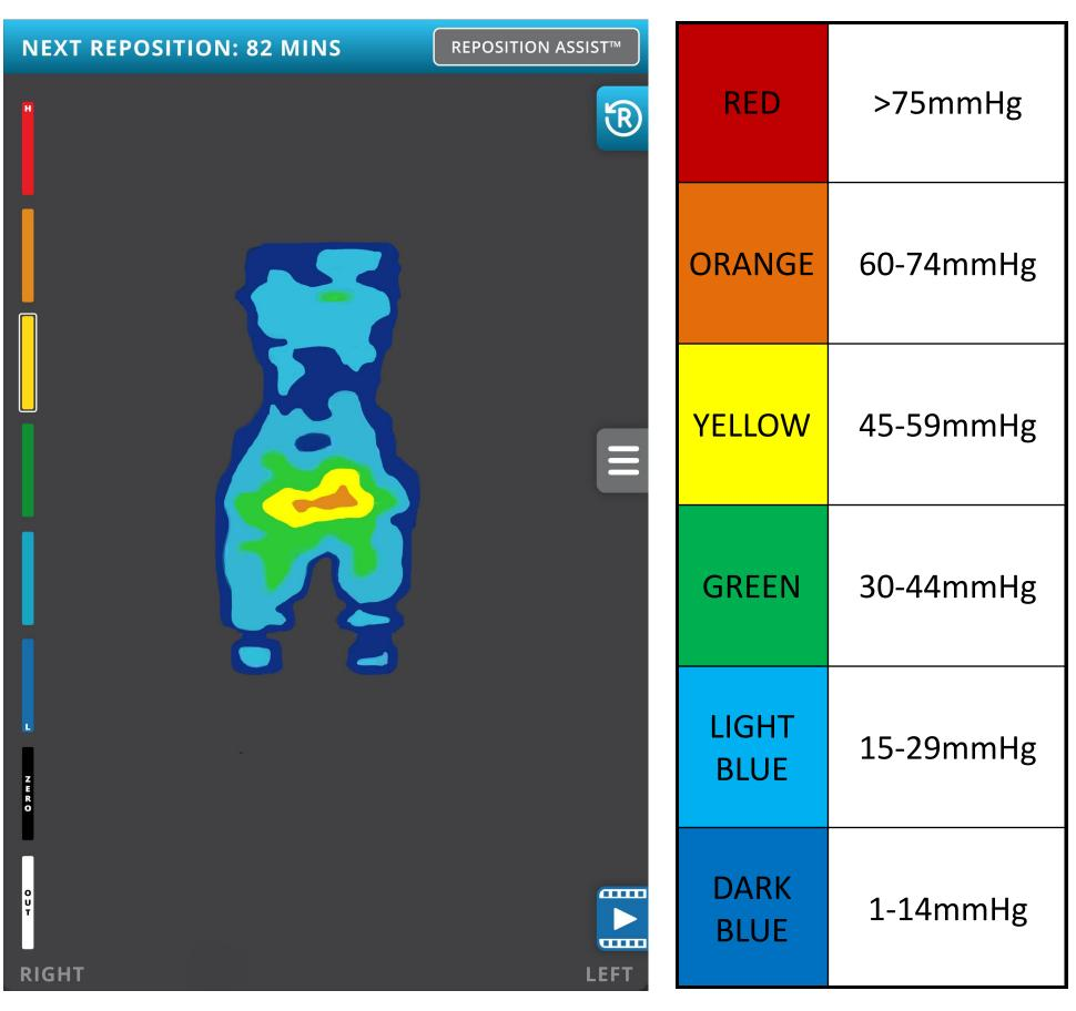
The APV pressure sensor mat and tablet were installed on 10 beds, displaying their body image with continuous pressure readings. Utilizing a color gradient to exhibit pressure values, patients were educated on the significance of each color in the gradient related to high - low pressure.
